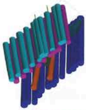
360° 3-D view created with Bauer's ABG software for high-level quality control and assurance
