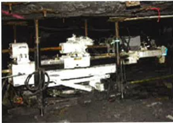
A long-hole directional drill used for in-mine CMM development Photo: REI Drilling
