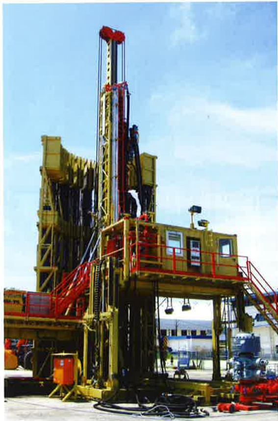
A Drillmec HH75 CBM rig in use in Indonesia
