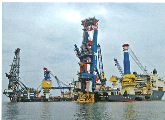
Saipem FDS-2 ship alongside FDS in operation at the Usan project in Nigeria
