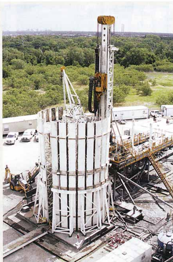
Fig. 5. The small footprint and low profile of these rigs makes them unobtrusive when used near urban areas.
