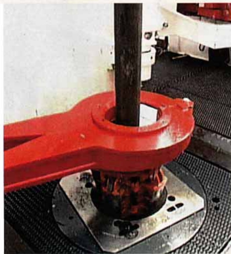
Fig. 4. Automated power tongs and hydraulic-powered slips are controlled from a cabin and are an essential part of a fully automated rig.
