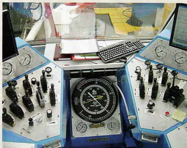
Fig. 1. The driller's cabin can control virtually all aspects of the automated drilling process.
