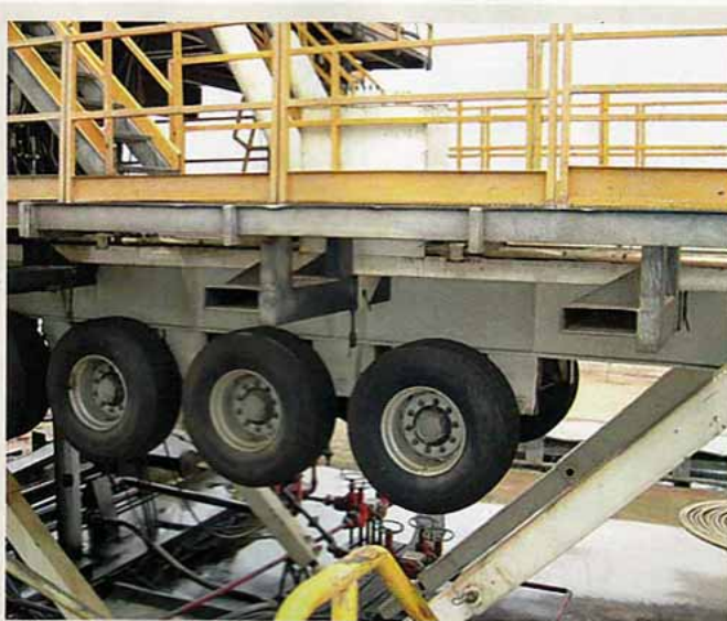
Fig. 2. The rig and its integral trailer are raised by a set of pistons.
