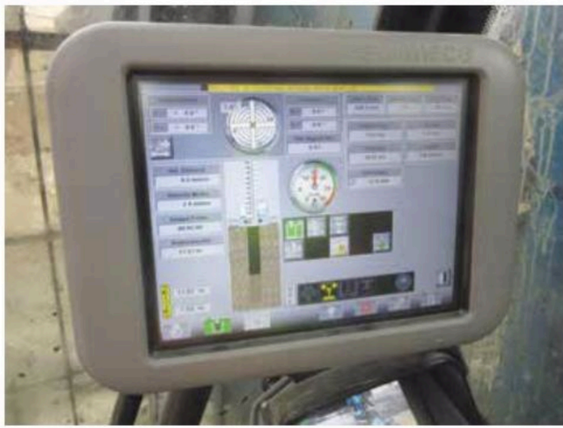
Above: The SR-45 is equipped with the Soilmec DMS system in order to have total control over the rig performance and site production rates.
